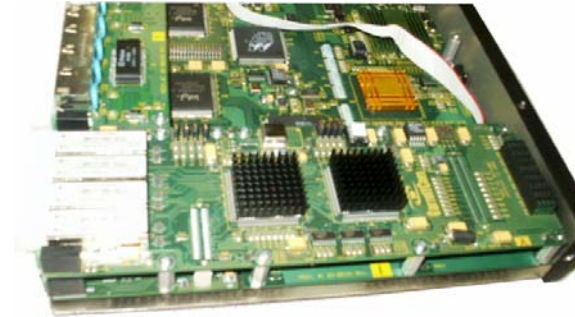
Fig. 3.5.2g Top View : 6KPM Module installed inside a 6K32 Switch
